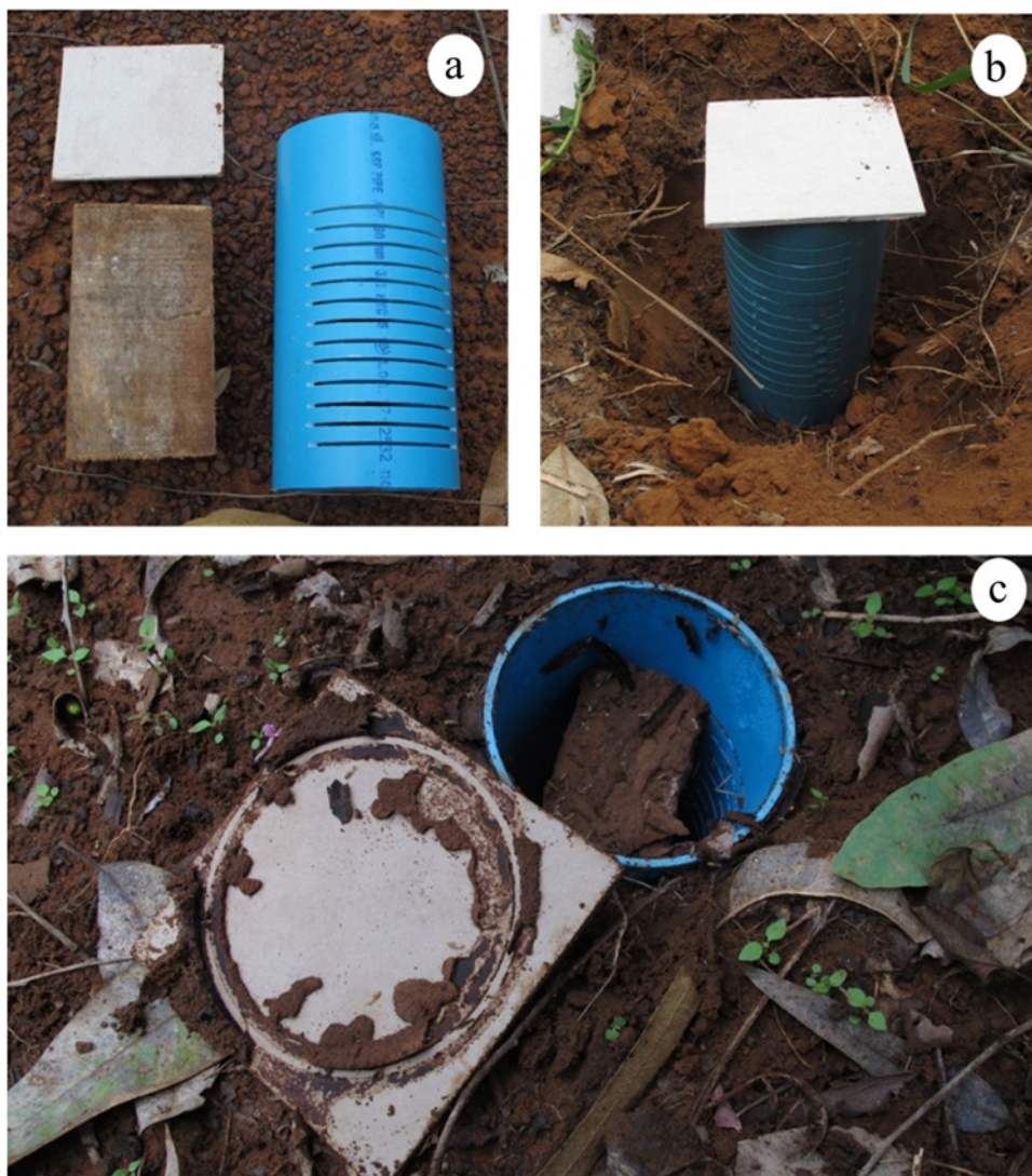
Figure 1. Subterranean termite baits were made by using (a) a PVC tube, rubber wood of dimensions 7.5 cm × 14 cm and a gypsum sheet. (b) Subterranean termite baits were buried in the soil and covered by a gypsum sheet, and (c) it was set up in the ground for 30 days.
