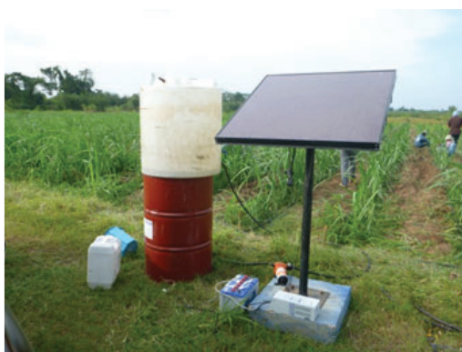
Figure 3 System design of drip irrigation powered by solar cell for rainfed sugarcane field in dry area with no electricity.
