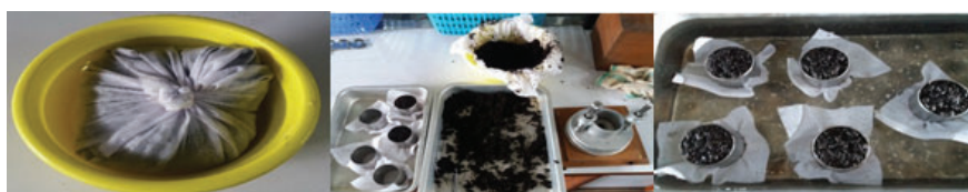
Figure 2 Growing substrate were compacted with cores by gravimetric method after that saturated with water for 1 hour.
