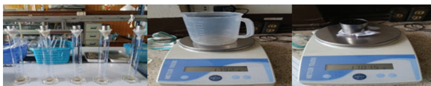
Figure 3 Measurement the amount of drained water and the weight of drained growing substrate to calculate for the field capacity (FC).
