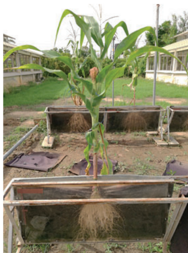
Figure 2 Overview of Rhizotron system in the experimental field and corn growing in soil-filled Rhizotron.
