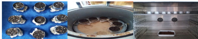
Figure 4 Calculation for permanent wilting point (PWP) by compressing the growing substrate in the 15 atmospheres condition until finishing of the draining. Then, the samples were dried up at 60°C for 3 days.
