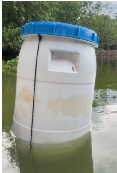
Figure 3. Field deployment of the smart water sampling buoy in a swamp environment during performance testing.
