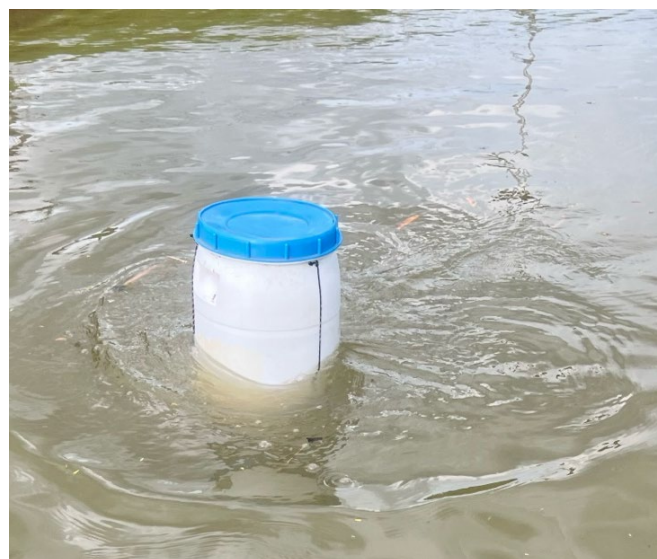
Figure 4. Field deployment of the smart water sampling buoy in a canal with moderate flow conditions.
