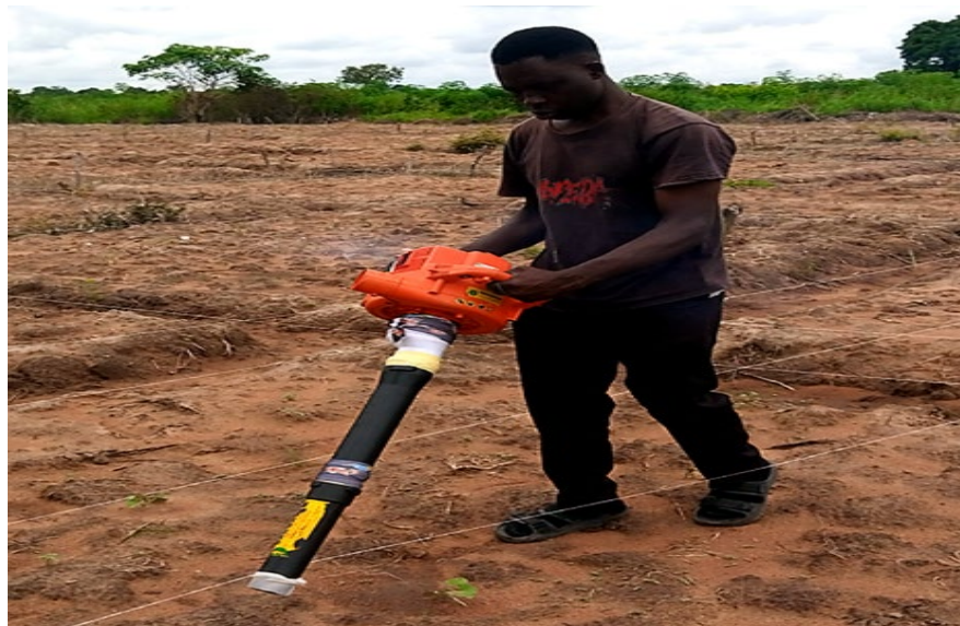
Figure 2. Arthropod suction sampling on golden melon plots using a modified Bragadin Giardinaggio portable 2-stroke gasoline-powered leaf-blower and vacuum machine during the 2025 cropping season at Wukari.
