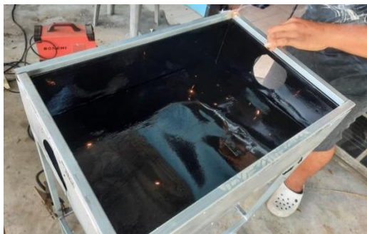
Figure 1. Inside of the automatic solar drying cabinet
