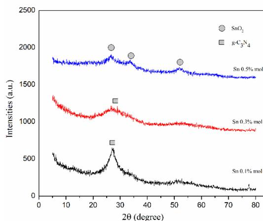
**Figure 7.** XRD patterns of the g-C<sub>3</sub>N<sub>4</sub> powder with various amounts of Sn doping.
