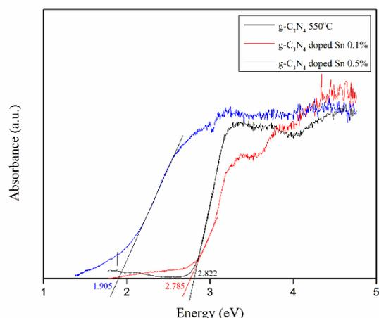
**Figure 9.** bandgaps of g-C<sub>3</sub>N<sub>4</sub> with difference doped Sn.
