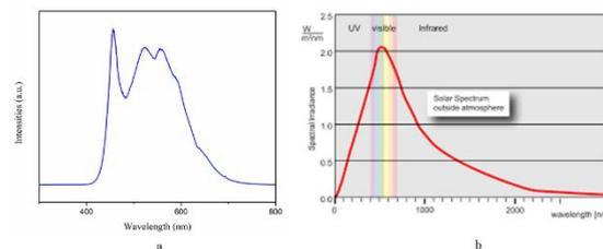
**Figure 11.** Light source spectrum (a) LED spectrum and (b) solar spectrum.
