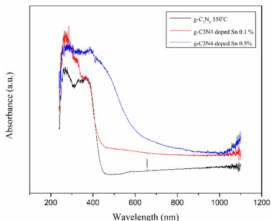
**Figure 8.** Light absorbance of g-C<sub>3</sub>N<sub>4</sub> powder with various amounts of Sn doping.
