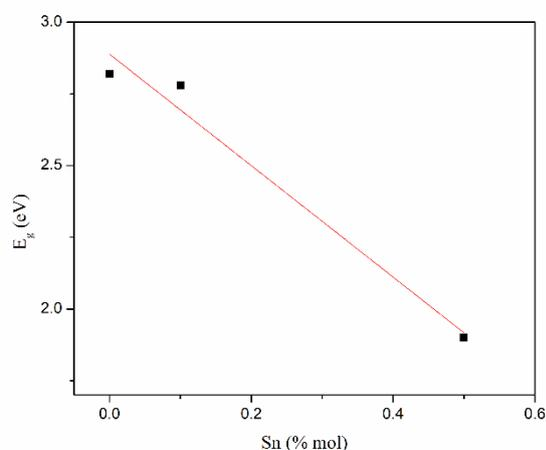
**Figure 10.** E<sub>g</sub> of Sn doped g-C<sub>3</sub>N<sub>4</sub> powders
