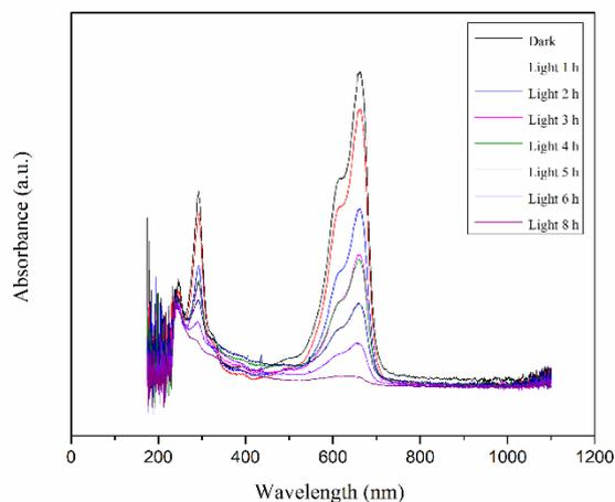
**Figure 15.** The light absorption of Sn-doped  $g-C_3N_4$ .
