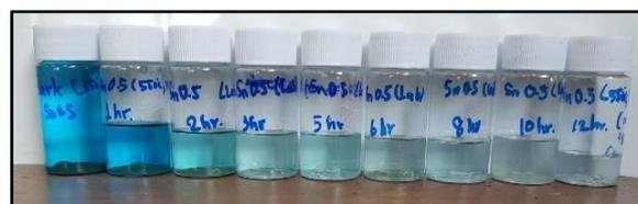
**Figure 17.** The degradation of MB of Sn-doped  $g-C_3N_4$ .
