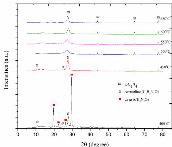
**Figure 1.** XRD patterns of the g-C<sub>3</sub>N<sub>4</sub> powders calcined at temperatures of 400-650°C.
