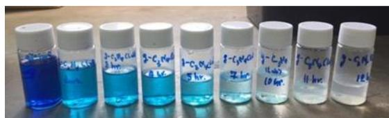
**Figure 14.** The degradation of MB of  $g-C_3N_4$ .
