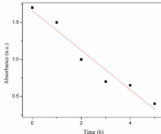
**Figure 16.** The light absorption at various times of Sn-doped  $g-C_3N_4$ .
