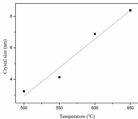
**Figure 2.** The relationship of g-C<sub>3</sub>N<sub>4</sub> crystal sizes to calcination temperatures.
