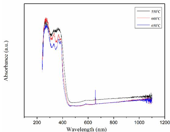
**Figure 3.** Light absorbance of g-C<sub>3</sub>N<sub>4</sub> powders at different calcination temperatures.
