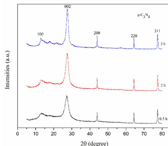
**Figure 4.** XRD patterns of the g-C<sub>3</sub>N<sub>4</sub> powder at various soaking times.
