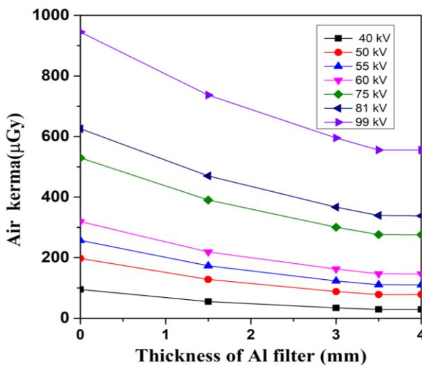
**Figure 3.** Graphical representation of dose as function of thickness for HVL measurements of Machine 4 (Siemens part8375545g2107) for 40, 50, 55, 60, 75, 81 and 99 kV respectively.
