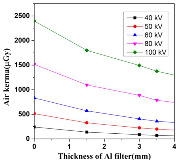
**Figure 2.** Graphical representation of dose as function of thickness for HVL measurements of Machine 1 (Shimadzu IEC60601-1-2-2001) for 40, 50, 60 80 and 100 kV respectively.
