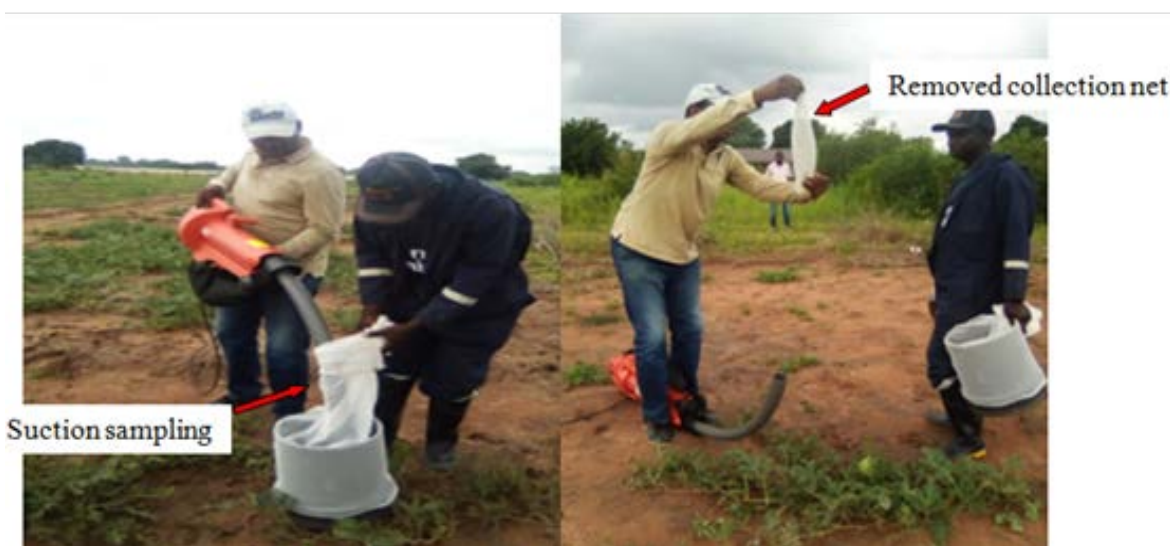
Figure 5. Suction sampling procedure.
