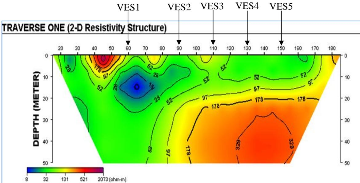
Figure 9. 2-D resistivity structure of traverse one
