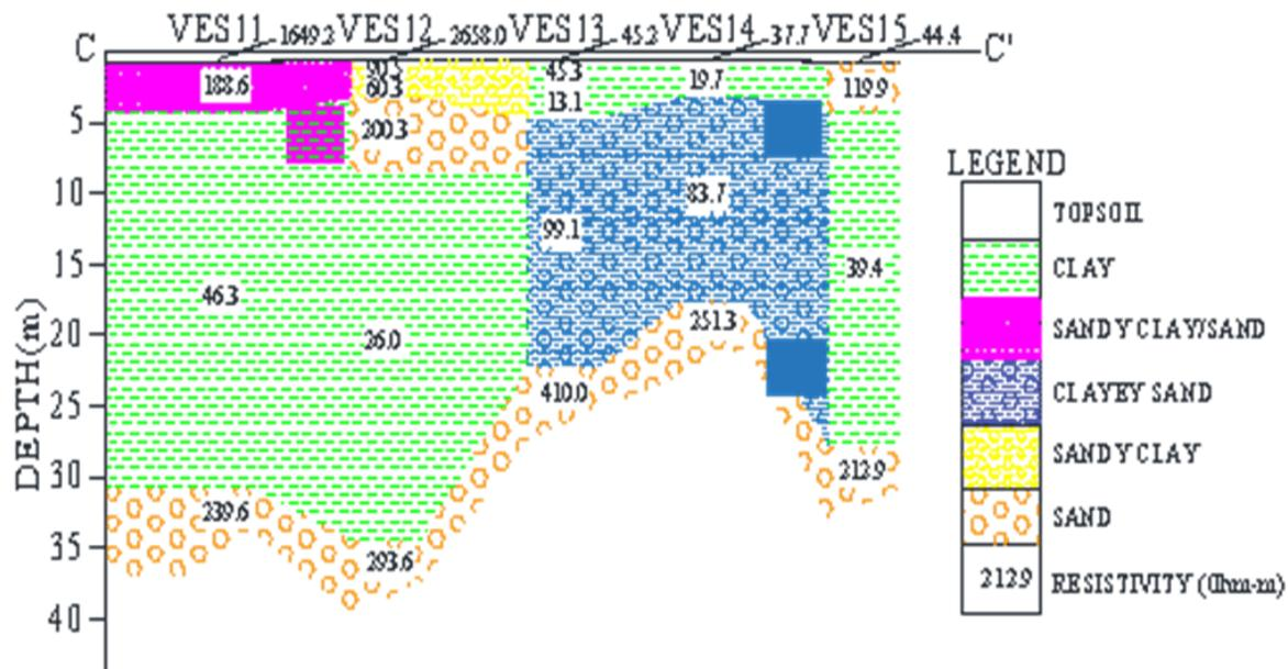
Figure 6. Geoelectric section for VES 11, 12, 13, 14 and 1
