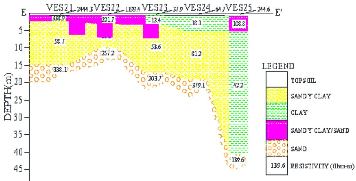
Figure 8. Geoelectric section for VES 21, 22, 23, 24 and 25.
