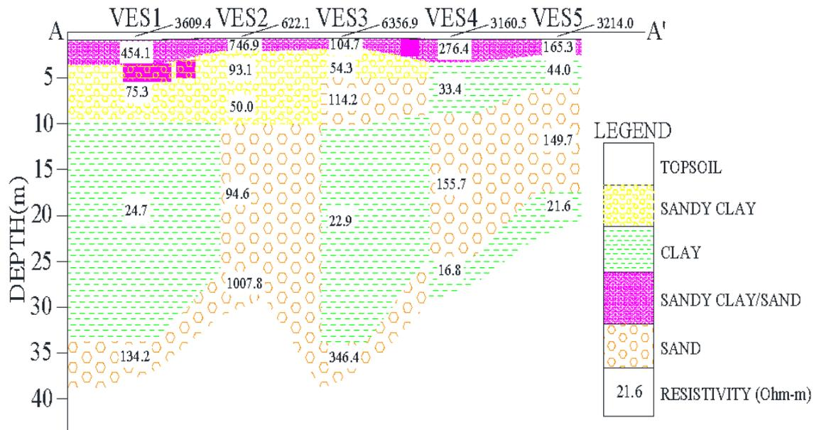
**Figure 4.** Geoelectric section for VES 1, 2, 3, 4 and 5.
