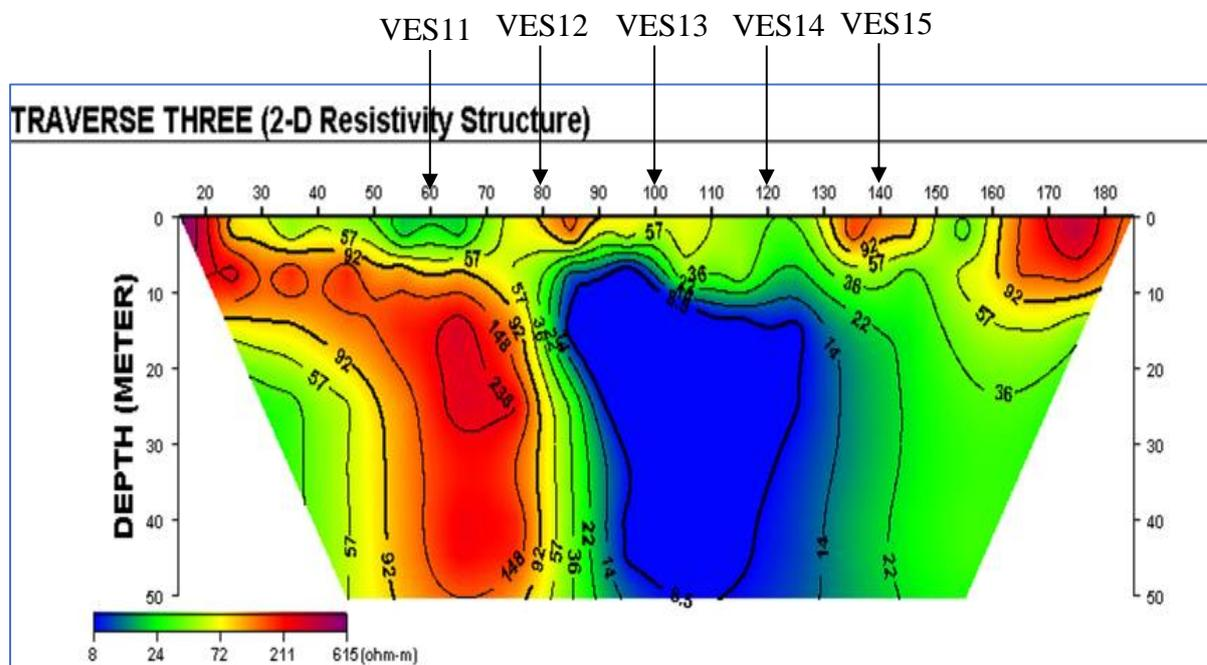
Figure 11. 2-D resistivity structure of traverse three.
