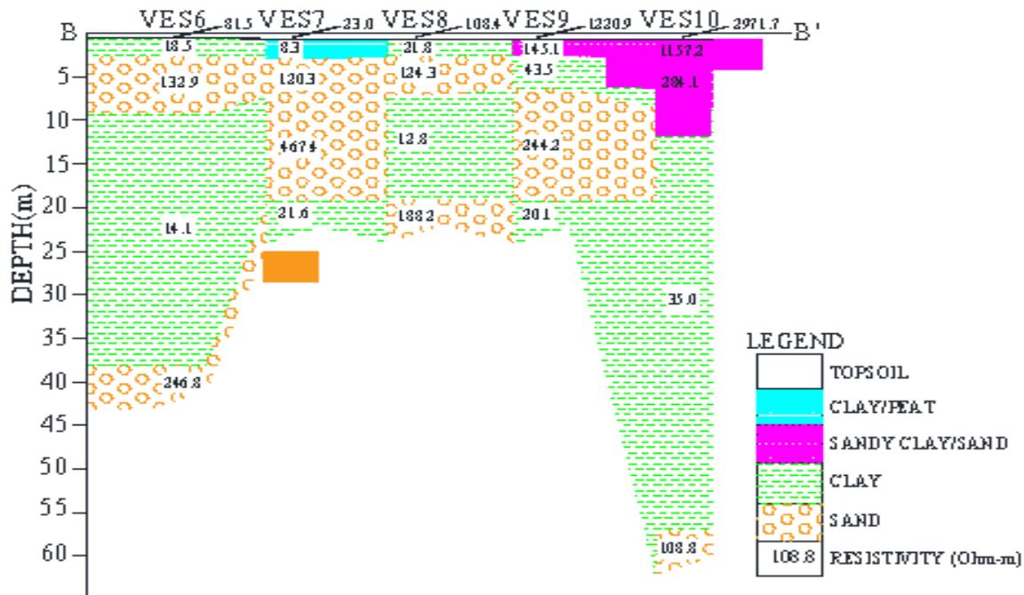
Figure 5. Geoelectric section for VES 6, 7, 8, 9 and 10.
