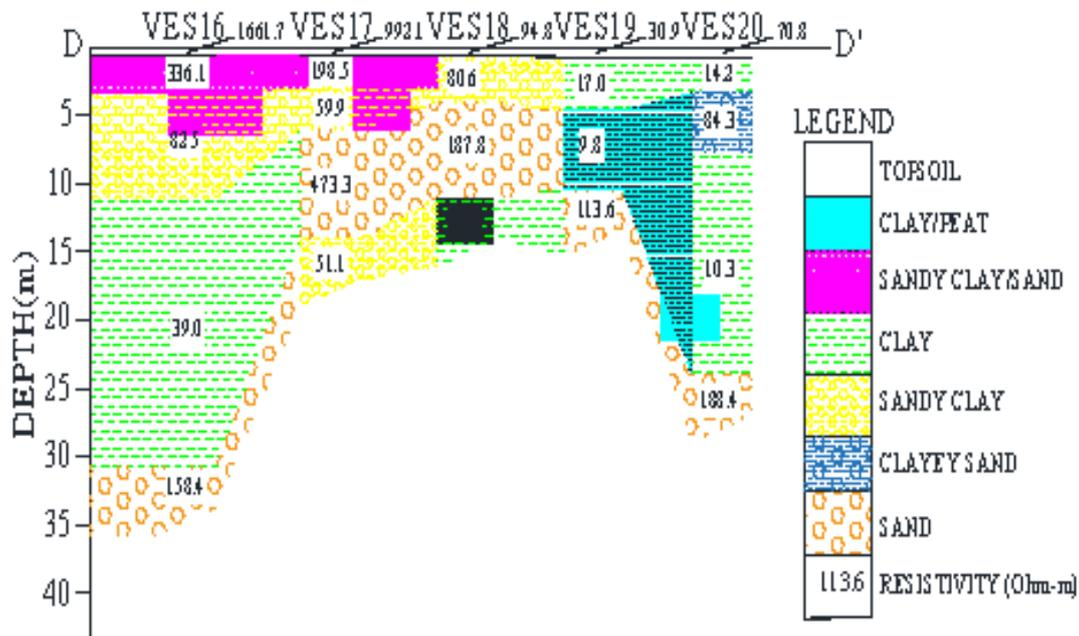
Figure 7. Goelectric section for VES 16, 17, 18, 19 and 20.
