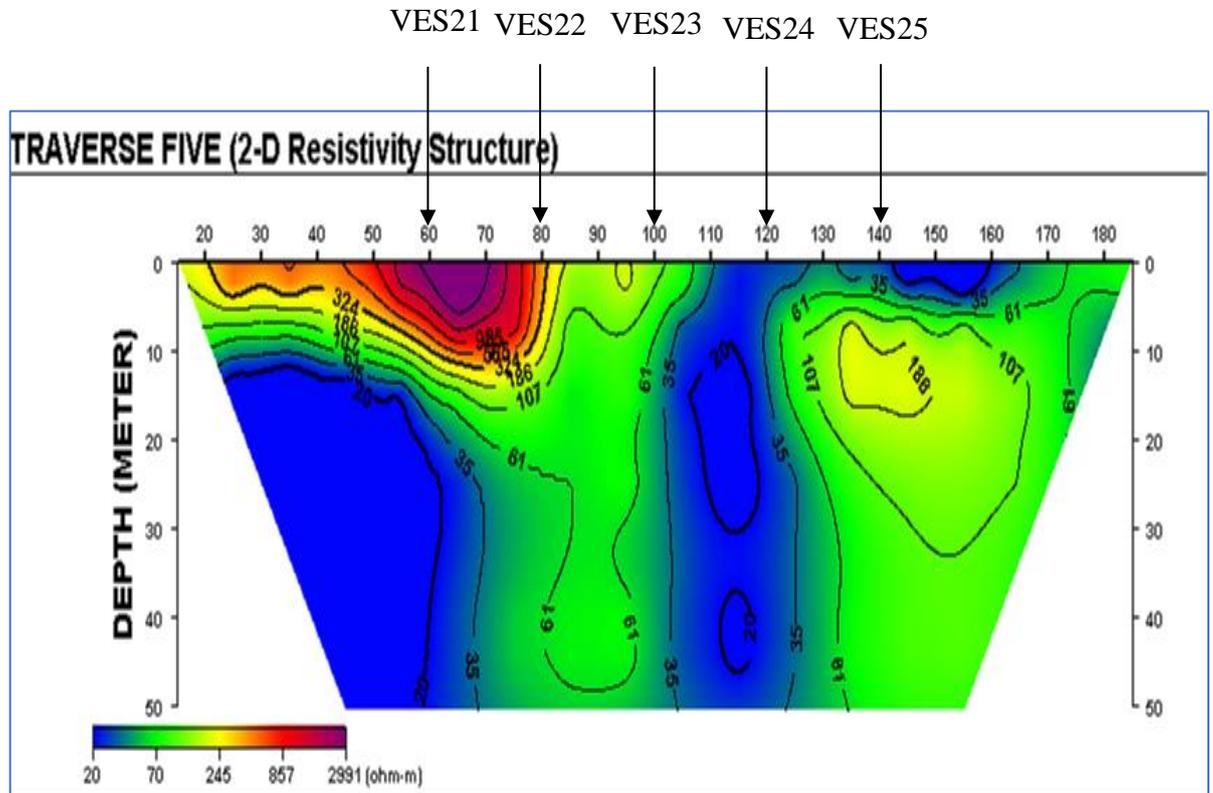
Figure 13. 2-D resistivity structure of traverse five.
