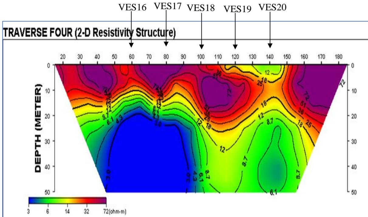
Figure 12. 2-D resistivity structure of traverse four.
