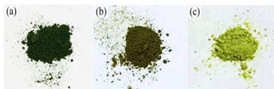
Figure 5. Colors of Co(8hq) 2 (a), MCM_Co(8hq) 2 (b) and MCMCo(II)_8hq (c)
