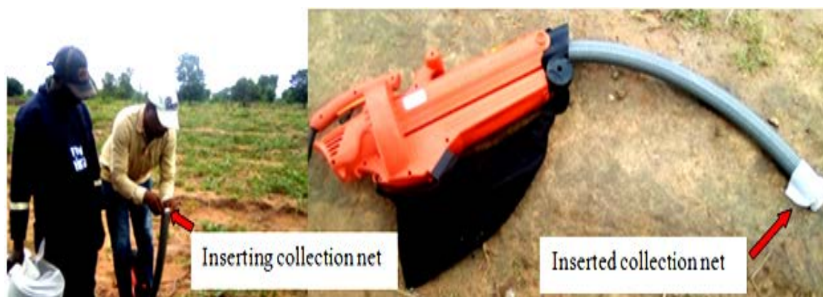
Figure 4. Insertion of the collection net into the intake nozzle, and the inserted collection net.
